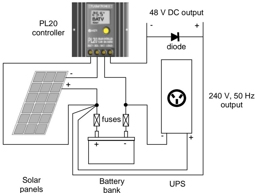
The diode is supplied with the PL20 and is used to protect the PL20. I used 15 Amp fuses on the battery, both positive and negative terminals, this would allow a maximum load of approximately 750 Watts. Its a bit conservative as the inverter is rated at 1500 Watts and they could be 25 amp. It means the load should not exceed 750 Watts if you don't want the fuses to blow.
